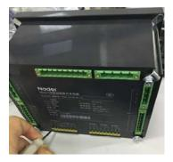
Two groups of yellow wiring card slots underneath in the figure above are secondary wiring terminals provided to customers with the wiring terminal functions shown as below:
