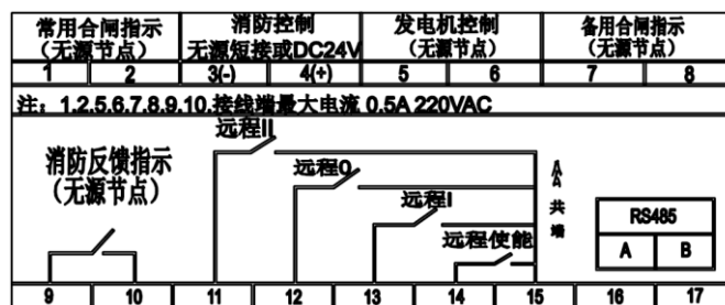
Fig. 6 (Type B controller) Secondary terminal wiring diagram
